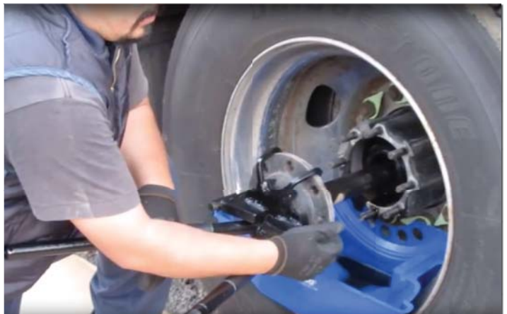
Carrillo demonstrates the EZ Axle Installer, which he designed.
